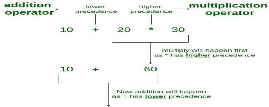
Figure 11 Example of Operator Precedence
