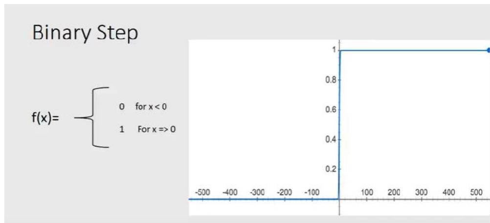
Figure 4 Binary step activation function
