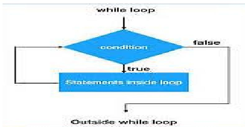
Figure 16 Flow chart of While Loop
